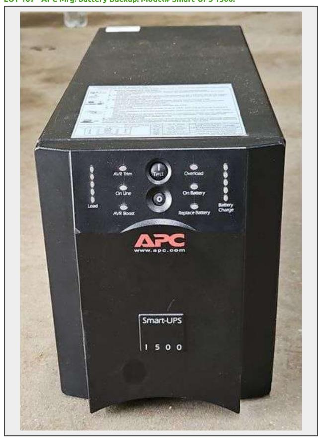
APC Battery Backup. Model# Smart-UPS 1500. 120V, 50/60Hz, 670Watts. Measures 16 1/2"x6 1/2"x8 1/2"
